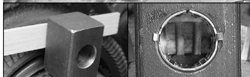
Block Mounting Reverse-A-Matic Sensor Mounting Diagrams Sensor Alignment, Outward ABS Ring Alingment Sensor Gap
