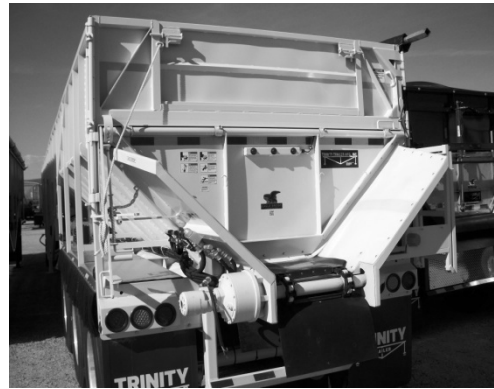
Figure 82 - Full Swing "Spud" With Manual Flip-Up Door
