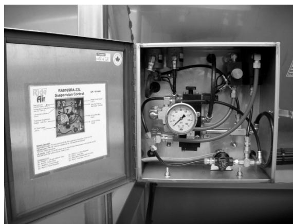
Figure 65 - RA016SRA-32L Suspension Control
