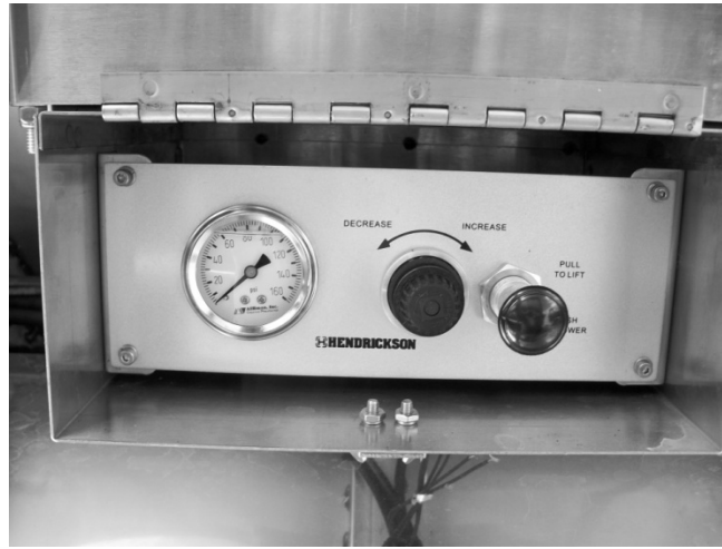
Figure 69 - HAC - USO/LSO Lift Control
