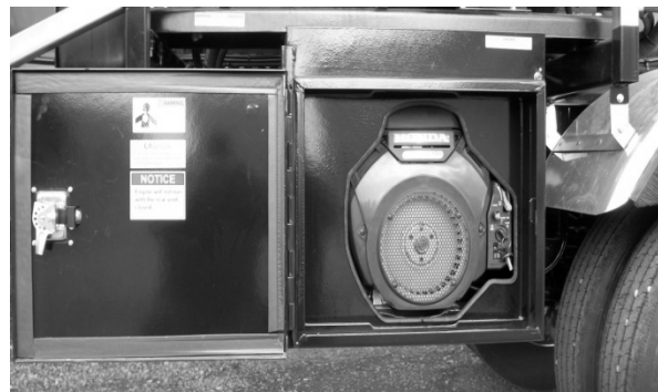
Figure 101 - 20 HP Gas Engine (Shown in Optional Enclosure)
