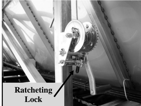
Figure 121 - Fold-Down Sideboard Door Operator Winch
