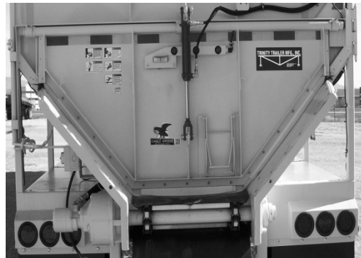
Figure 76 - Hydraulic Flip-Up Lower Door
