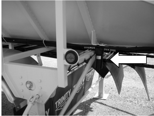
Figure 40 - Pressure Filter Location
