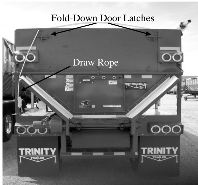
Figure 92 - "Spud" Door Components
