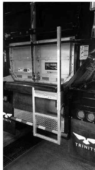
Figure 153 – Ladder "In-use" position
