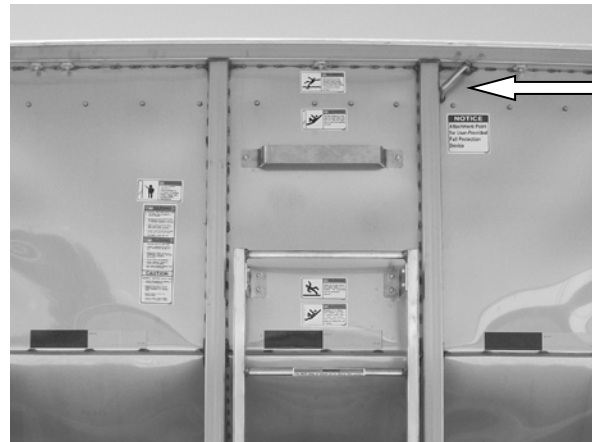
Figure 149 - User Fall Protection Device Attachment Point
