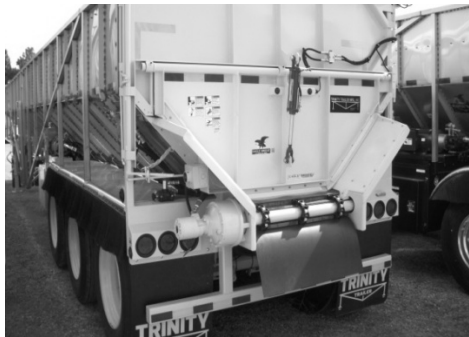
Figure 85 - Full Swing With Hydraulic Flip-Up Door
