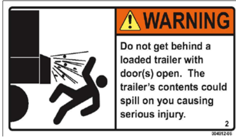
Figure 113 - Getting Behind Trailer Decal
