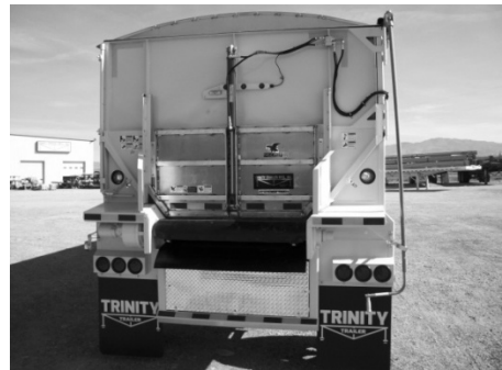
Figure 86 - Full Swing With Hydraulic Slide-Up Door
