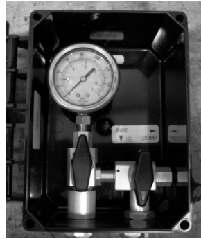
Figure 53 - Dump valve used with air gauge
