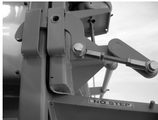
Figure 98 - Top Hinge Pneumatic Latch Disengaged
