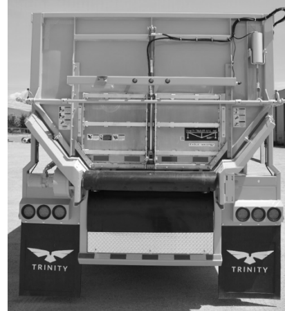
Figure 90 - Hydraulic Lift Top-Hinge with Hydraulic Slide-Up Door
