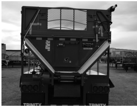
Figure 83 - Full Swing "Spud" With Hydraulic Flip-Up Door
