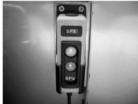
Figure 108 - DC Hydraulic Control Unit
