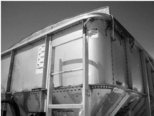
Figure 146 - Front Ladder Showing Upper User Fall Protection Device
