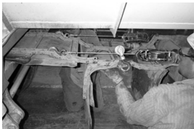
Figure 7 - Determine How Much Chain to Remove
