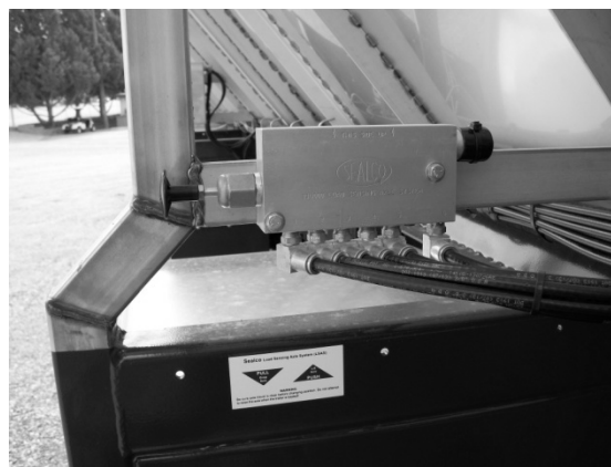
Figure 62 - LSAS Lift Control
