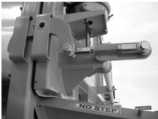
Figure 97 - Top Hinge Pneumatic Latch Engaged
