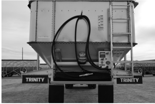
Figure 126 -Pneumatically-Actuated Front Wet Seal
