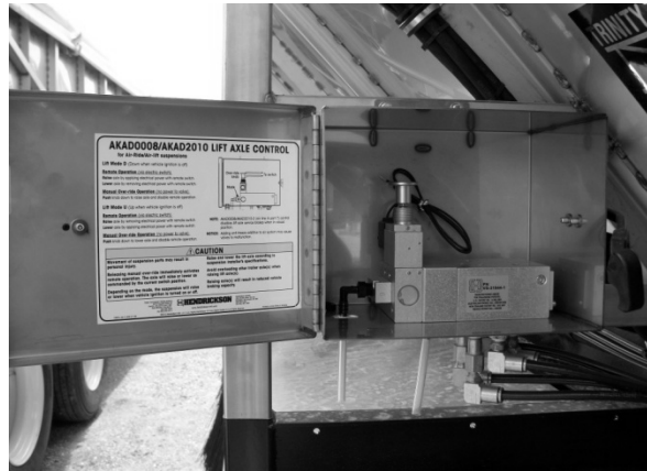
Figure 61 - AKAD2010 Lift Control
