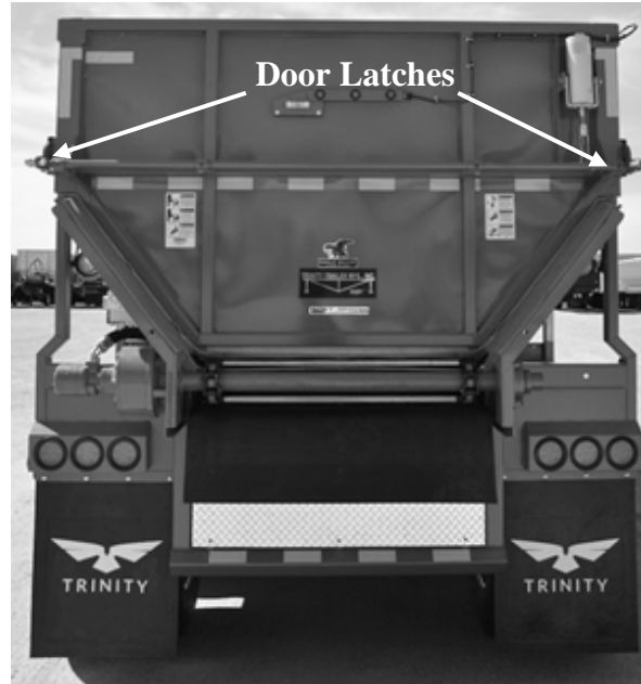
Figure 96 - Top Hinge Pneumatic Latches
