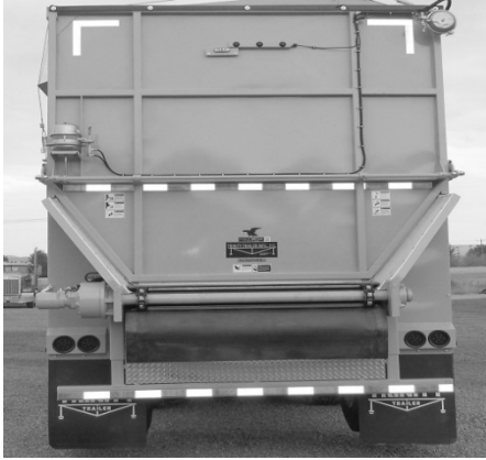
Figure 87 - Pneumatic Lift Top-Hinge with No Lower Door
