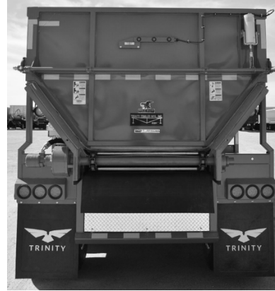
Figure 88 - Hydraulic Lift Top-Hinge with No Lower Door
