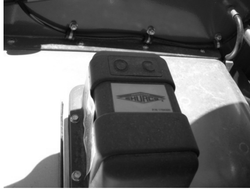
Figure 135 - Electric Tarp Rocker Switch
