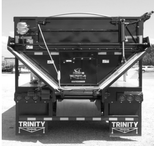
Figure 91 - Hydraulic Lift Top-Hinge "Spud" With Hydraulic Flip-Up Door
