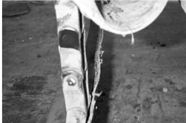
Figure 8 - Chain Pin with Head Ground Off
