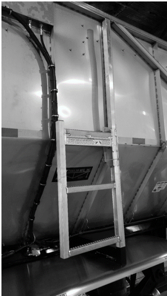
Figure 150 - Maintenance Ladder "Stowed" Position
