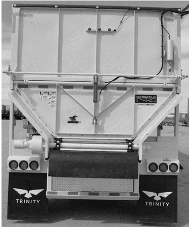
Figure 89 - Hydraulic Lift Top-Hinge with Hydraulic Flip-Up Door
