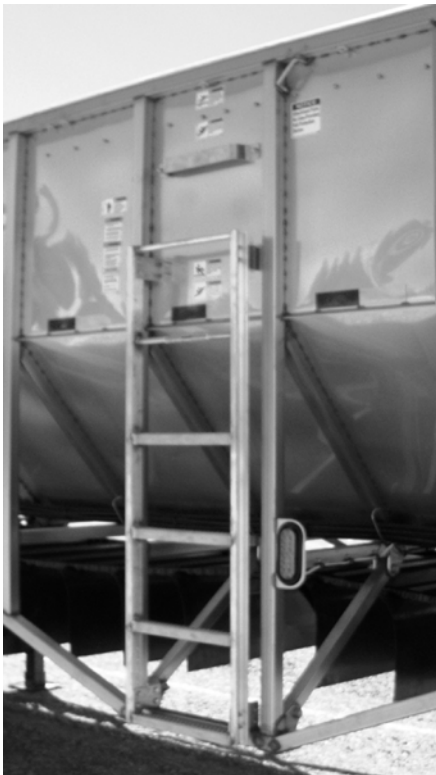
Figure 148 - Roadside Ladder Showing Offset
