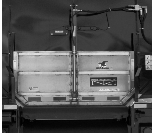
Figure 78 - Hydraulic Slide-Up Lower Door
