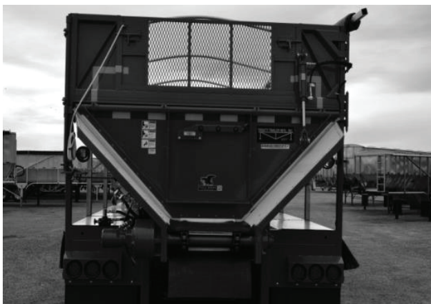
Figure 93 Full Swing “Spud” with Hydraulic Flip-Up Door
