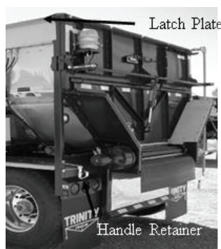
Figure 145 Shur-Lok® Roadside Hardware. Latch Plate: Part #004742
