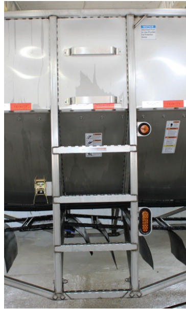
Figure 160 Road Side Ladder Showing Weld on Rungs
