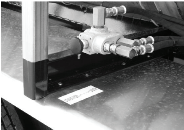
Figure 115 Push-Pull Valve Used to Select Door or Belt Control. Part #004894
