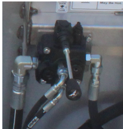
Figure 116 Single Door Valve for Door Control Part #003728
