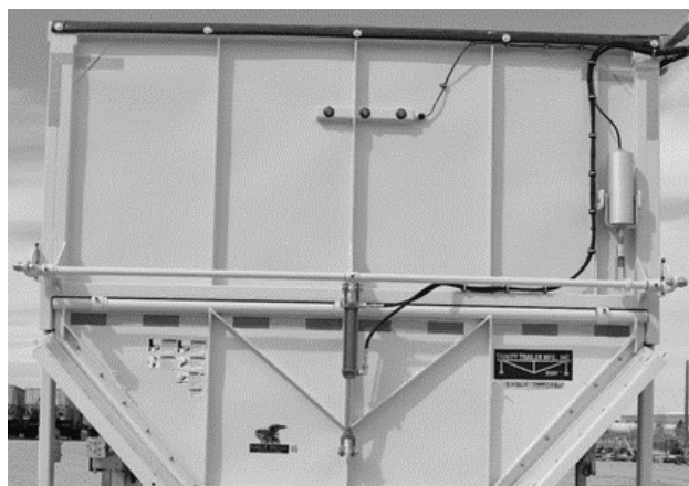
Figure 98 Hydraulic Top Hinge with Hydraulic Lower Flip-Up
