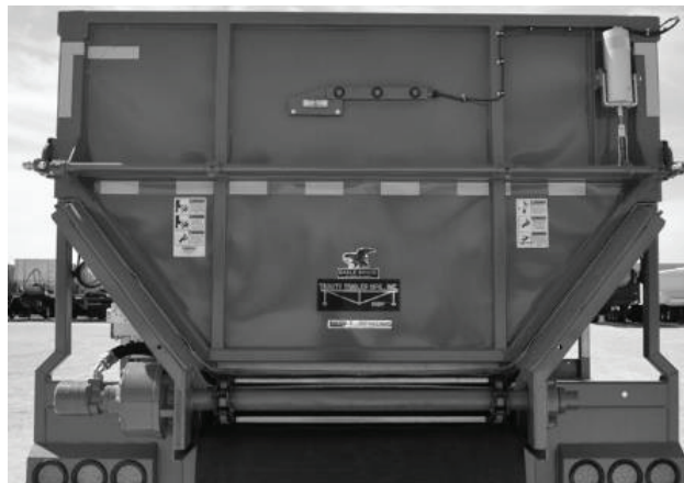
Figure 100 Hydraulic Top Hinge with No Lower Function
