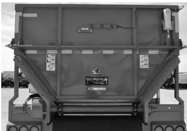
Figure 97 Hydraulic Top Hinge with No Lower Function
