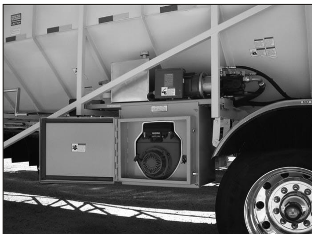
Figure 52- 20HP Gasoline Engine (Shown mounted in optional motor box)
