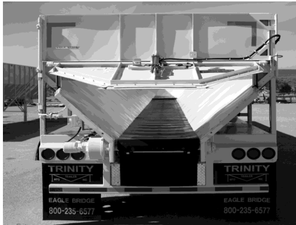
Figure 70-Full-Swing Door with Hydraulic Flip-Up Door
