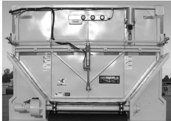
Figure 82-Top-Hinged Slider Door with Pneumatic Latches, Hydraulic Lift and Hydraulic Flip-Up Door
