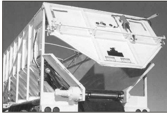
Figure 80-Top-Hinged Door with Pneumatic Latch and Hydraulic Lift
