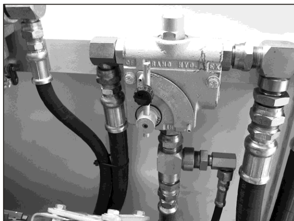
Figure 55- Flow Control Valve Used to Control Conveyor Speed with PTO Systems
