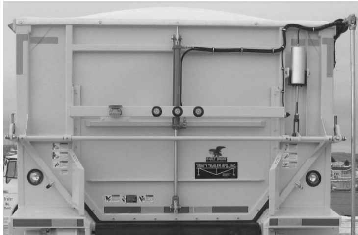
Figure 81-Top-Hinged Door with Pneumatic Latch, Hydraulic Lift and Hydraulic Slide-Up Door
