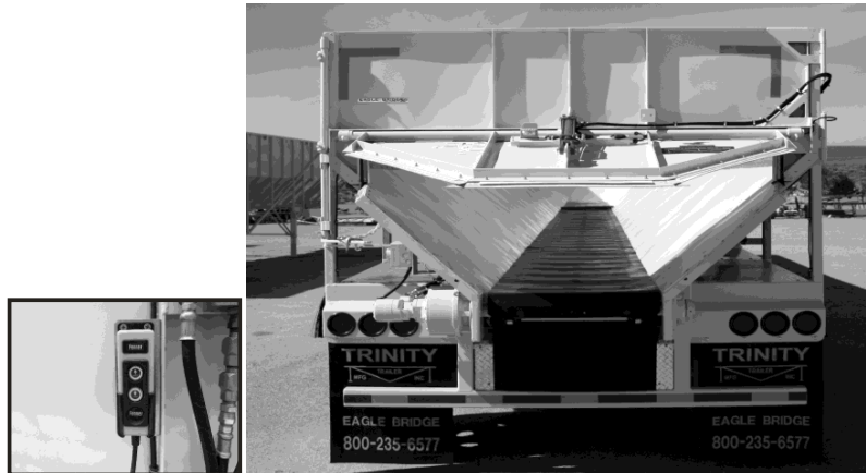
Figure 71 -Full-Swing Door with DC-Powered Hydraulic Flip-Up Door
