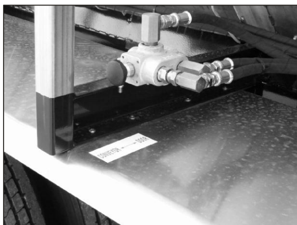
Figure 56- Push-Pull Valve Used to Select Door or Conveyor
