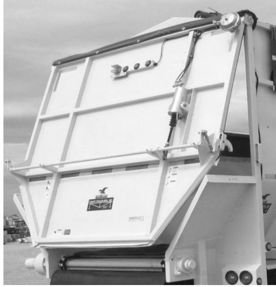
Figure 78- Top-Hinged Door with Pneumatic Latch and Pneumatic Lift
