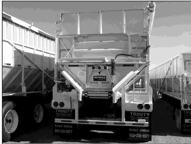
Figure 77 -Full-Swing “Spud” Door with Hydraulic Flip-Up Door
