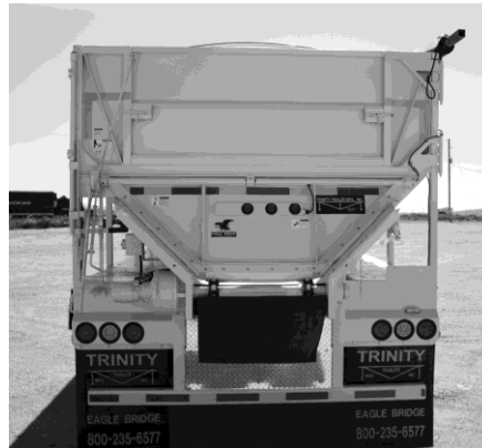
Figure 76 -Full-Swing “Spud” Door with Manual Flip-Up Door
