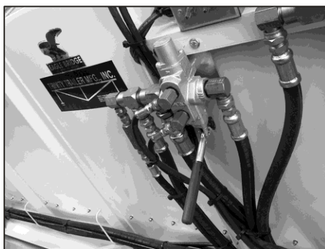
Figure 57a-Door Valve for Opening and Closing Door
