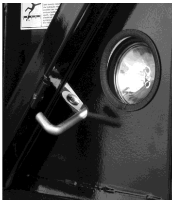
Figure 51- Top-Hinged Slide-Up Door Safety Latch
