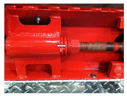
Figure 4 - Chain Adjustment
