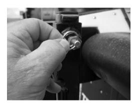
**Figure 153** - Telescoping Handle Release Pin
