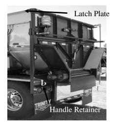
Figure 133 - Shur-Lok® Tarp Rolled Up
