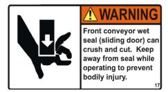
Figure 126 - Warning Label for Pneumatically-Actuated Front Wet Seal
