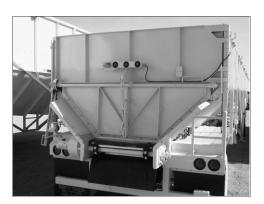
**Figure 85** - Full Swing With Manual Flip-Up Door
