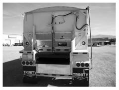
**Figure 87** - Full Swing With Hydraulic Slide-Up Door
