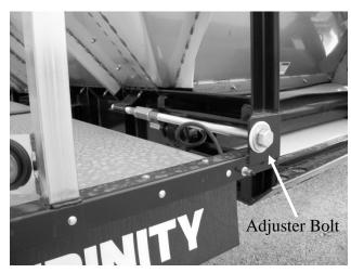
Figure 4 - Chain Adjustment Assembly
