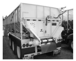
**Figure 86** - Full Swing With Hydraulic Flip-Up Door
