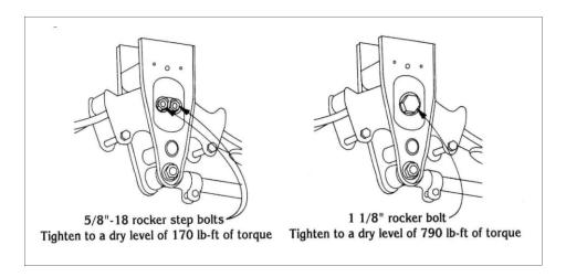
Figure 20 - Rocker Bushing Bolts
