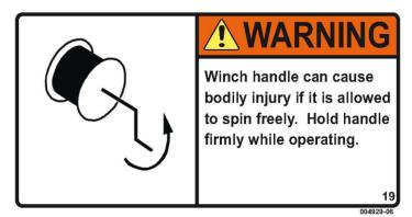
Figure 124 - Moving Winch Parts Decal
