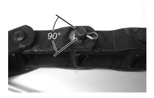
Figure 9 - Properly Welded Pin
