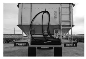
**Figure 127 -**Pneumatically-Actuated Front Wet Seal
