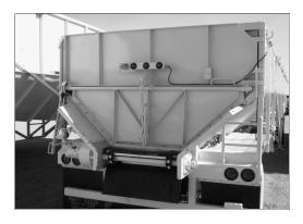
**Figure 76 -** Manual Flip-Up Lower Door
