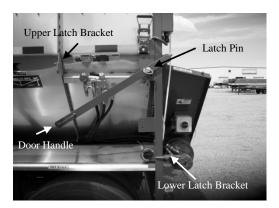
Figure 80 - Manual "Spud" Door Components
