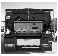
**Figure 91** - Hydraulic Lift Top-Hinge with Hydraulic Slide-Up Door
