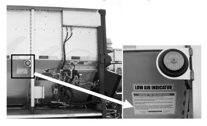
Figure 71 - Tire Inflation System Indicator Lamp
