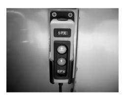
Figure 109 - DC Hydraulic Control Unit
