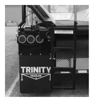
**Figure 156** - Maintenance Ladder In Use Position
