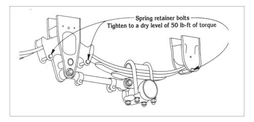
Figure 21 - Spring Retainer Bolts
