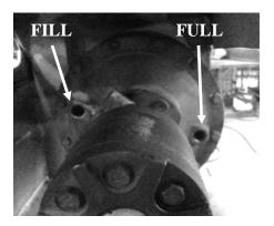
Figure 13 - Planetary Plugs
