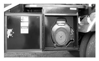
**Figure 102** - 20 HP Gas Engine (Shown in Optional Enclosure)
