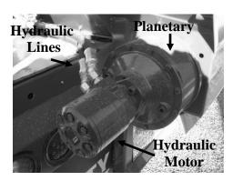
Figure 10 - Planetary
