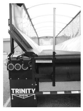
**Figure 155** - Telescoping Handle Extended
