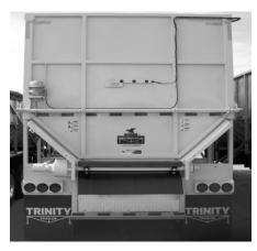
**Figure 89** - Hydraulic Lift Top-Hinge with No Lower Door
