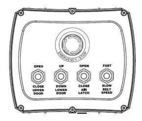
Figure 110 - Wired Remote Control Panel
