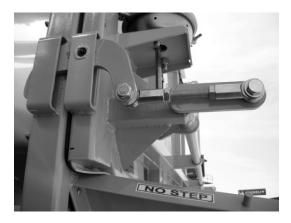
**Figure 98** - Top Hinge Pneumatic Latch Engaged
