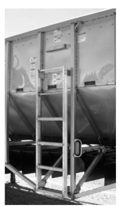
**Figure 149 -** Roadside Ladder Showing Offset
