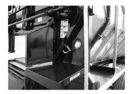
Figure 101- Slide-Up Door Clamp Latch Disengaged
