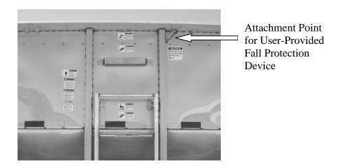
Figure 150 - User Fall Protection Device Attachment Point
