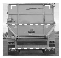
**Figure 88** - Pneumatic Lift Top-Hinge with No Lower Door
