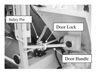
Figure 95 - Full-Swing Door Latch Components
