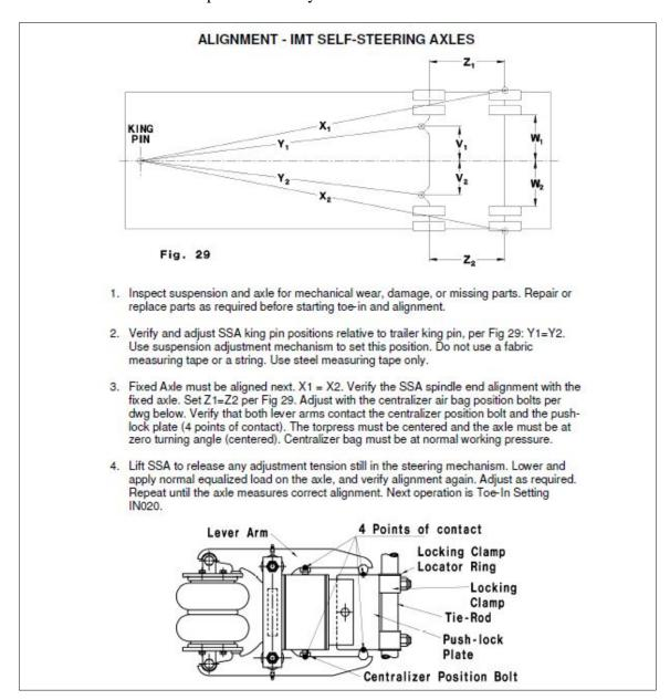
Figure 35 - IMT Self-Steering Alignment Procedure
