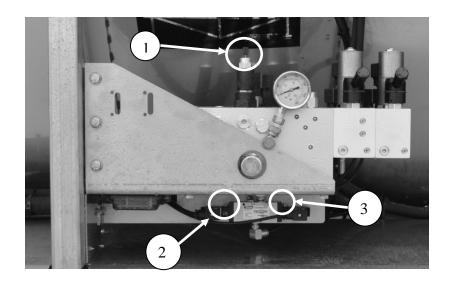
Figure 111 - Manifold with Solenoid Controls
