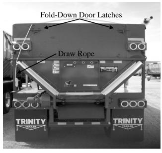
Figure 93 - "Spud" Door Components
