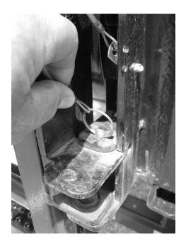
**Figure 152** - Position Locking Pin
