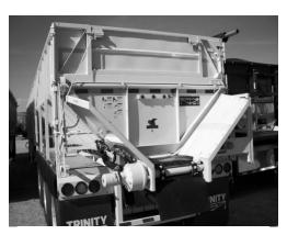
**Figure 83** - Full Swing "Spud" With Manual Flip-Up Door
