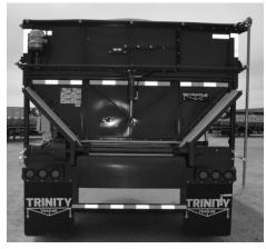
**Figure 90** - Hydraulic Lift Top-Hinge with Hydraulic Flip-Up Door
