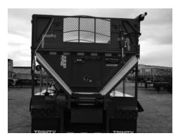
**Figure 84** - Full Swing "Spud" With Hydraulic Flip-Up Door
