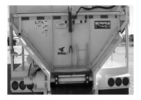
**Figure 77 -** Hydraulic Flip-Up Lower Door
