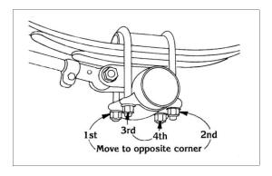
Figure 18 - Spring Suspension Axle Clamp Tightening Sequence
