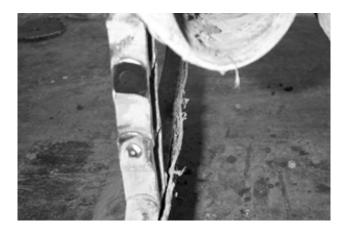
Figure 8 - Chain Pin with Head Ground Off
