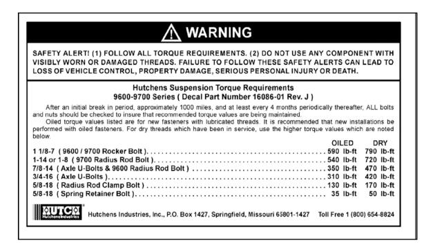
Figure 17 - Spring Suspension Torque Requirements
