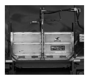
**Figure 79** - Hydraulic Slide-Up Lower Door
