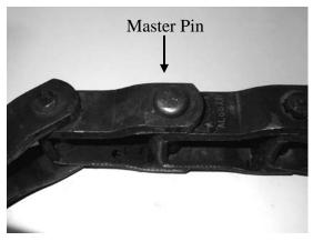
Figure 5 - Master Pin Identification
