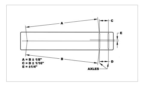
Figure 23 - Suspension Alignment Requirements
