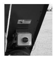
Figure 104 - Electric Motor Power Switch
