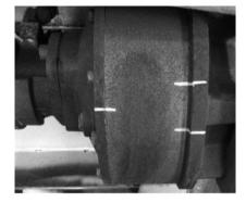
Figure 11 - Planetary Position Marking
