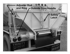
Figure 81 - Manual Flip-Up Door Components
