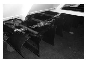
Figure 6 - Using Come-Along To Pull Up Chain Slack
