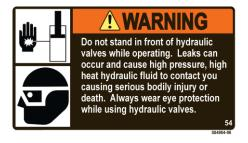
Figure 119 - Hydraulic Valve Decal
