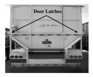
**Figure 97** - Top Hinge Pneumatic Latches
