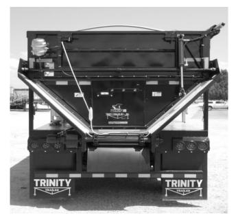
**Figure 92** - Hydraulic Lift Top-Hinge "Spud" With Hydraulic Flip-Up Door
