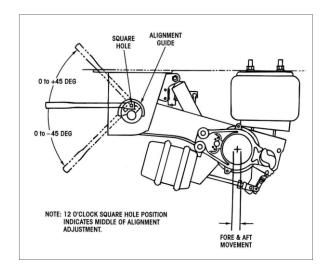
Figure 31 - Air-ride Suspension Alignment
