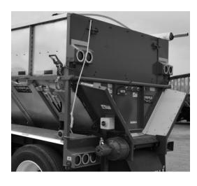
Figure 78 - Manual "Spud" Lower Door
