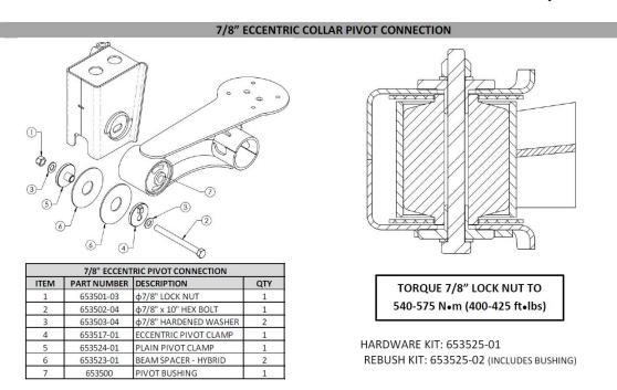
Figure 33 - ISS Series Eccentric Collar Components
