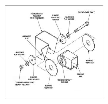
Figure 30 - Air-ride Suspension Alignment Components
