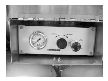
Figure 69 - HAC - USO/LSO Lift Control
