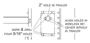
**STEP 3:** Install grommet into 2" hole. Insert wire from wireless receiver through grommet.
