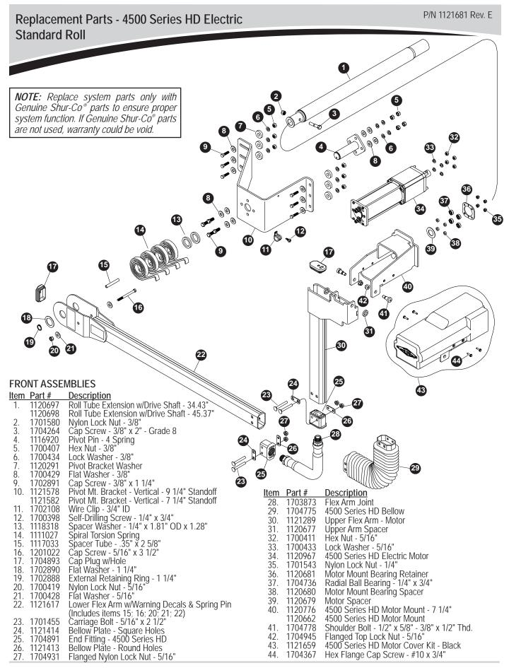
P/N 1121681 Rev. E Replacement Parts - 4500 Series HD Electric - continued **Standard Roll N**O .*o*° 0<sub>C</sub>
