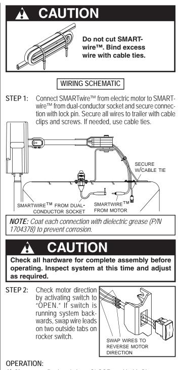
A) Close tarp: Push switch to "CLOSE" and hold. Observe tarp and release switch when tarp is fully closed.
