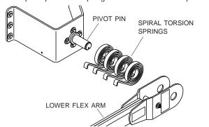
**STEP 8:** Secure with 1 1/4" flat washer and retaining ring.
