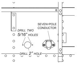
**STEP 2:** Align socket over 2" hole. Using holes in flanges on socket as guide, mark and drill two 5/16" holes.
