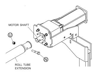
**STEP 4:** Hold flex arm with motor and roll tube extension in vertical plane to trailer and 90° to roll tube. Mark roll tube at location to be cut.
