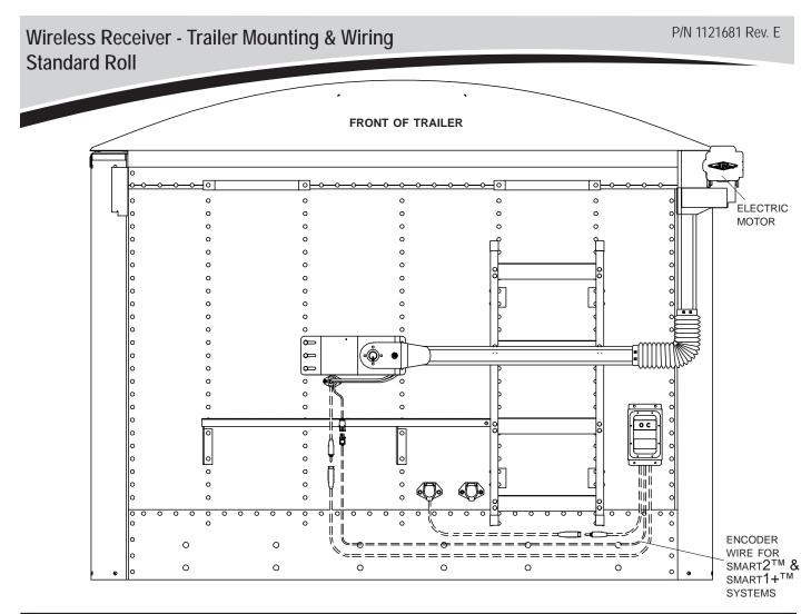
**NOTE:** Wire lengths are predetermined. Before installing SMARTwire<sup>™</sup> components, review and confirm wire routing so wires reach components with ample room for connection.
