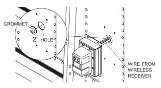
**STEP 4:** Align holes on wireless receiver with holes on trailer. Fasten receiver to trailer with 5/16" x 7/8" cap screws, lock washers and nuts.
