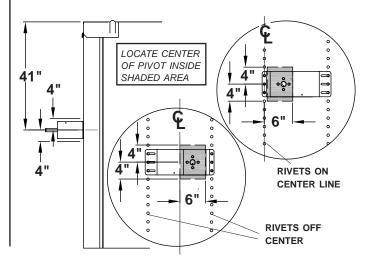
**NOTE:** Mount brackets into support braces on trailer, if possible. If bracket cannot be mounted into support braces, reinforce mounting area with backer plate for adequate support. Before drilling any holes, make sure flex arm has a clear pathway to operate.
