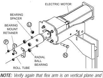
**NOTE:** Verify again that flex arm is on vertical plane and parallel to face panel before proceeding. Make sure all fasteners holding motor to upper flex arm bracket are tightened securely. **STEP 9:** Fasten motor cover onto motor with #10 x 3/4" screws.
