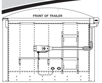
**NOTE:** Wire lengths are predetermined. Before installing SMARTwire<sup>™</sup> components, review and confirm wire routing so wires reach components with ample room for connection.
