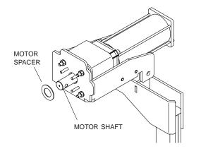
STEP 3B: Slide roll tube extension over motor shaft. Fasten with 3/8" x 2" cap screws and lock nuts. Finger tighten only.
