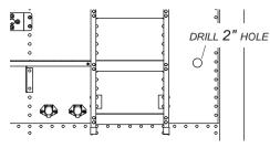
**STEP 2:** Align holes in wireless receiver over 2" hole in trailer as shown below. Using holes on flanges on receiver as a guide, mark and drill four 5/16" holes as shown.
