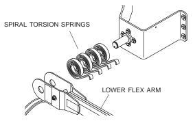
STEP 4: Secure with 1 1/4" flat washer and retaining ring.
