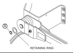
**NOTE:** Motor assembly on upper flex arm must face toward trailer as shown.
