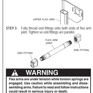
STEP 4: Insert flex arm joint into upper flex arm and slide bellow over flex arm joint. Align holes in upper flex arm, bellow plates, flex arm joint and bellow. Fasten with 5/16" carriage bolts and flanged nylon lock nuts.
