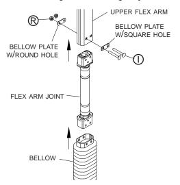
STEP 5: Insert lower end fitting into lower flex arm assembly with end of bellow over outside of arm. Align holes in lower flex arm assembly, bellow plates, end fitting and bellow. Fasten with 5/16" carriage bolts and flanged nylon lock nuts.
