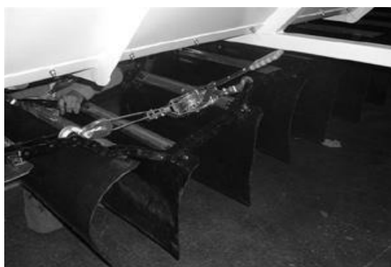
Figure 6 - Using Come-Along To Pull Up Chain Slack
