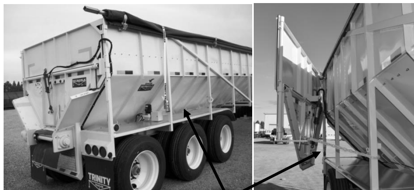
Figure 100- Full Swing Door Latch Components
