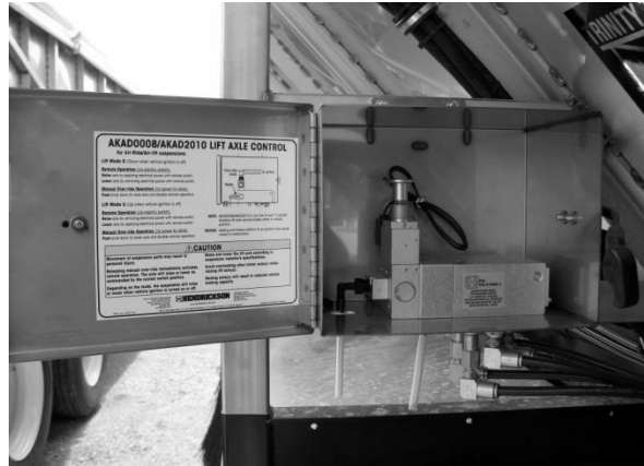
Figure 69- AKAD2010 Lift Control - Part #004230
