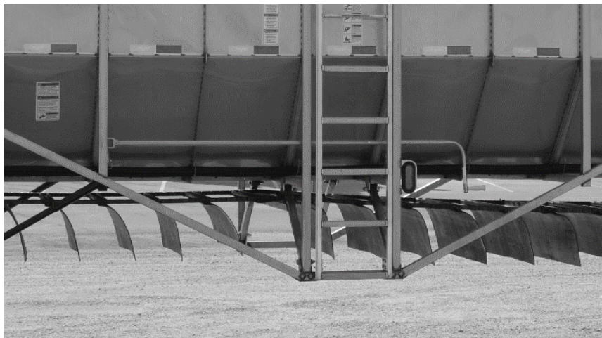
Figure 142- Rollover Tarp Handle Stored.
