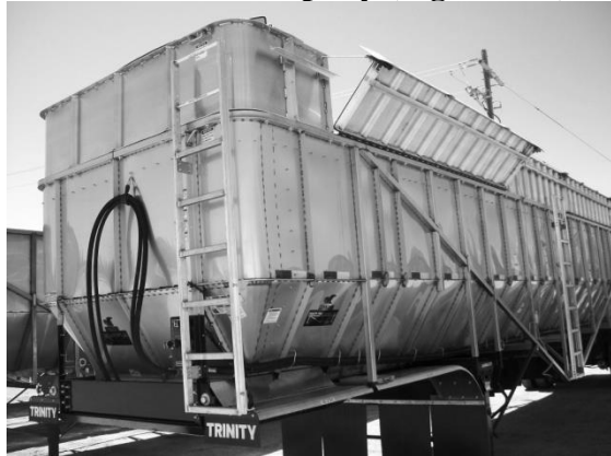
Figure 131- Fold-Down Sideboard Door
