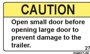
Figure 123 - Door Opening Sequence
