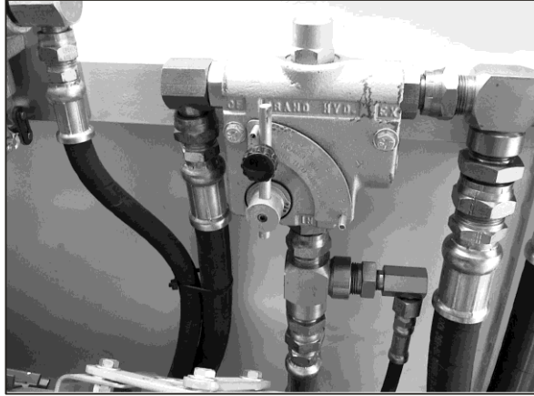
Figure 111- Flow Control Used to Control Belt in PTO Systems. - Part #004402
