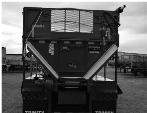
Figure 93- Full Swing "Spud" with Hydraulic Flip-Up Door
