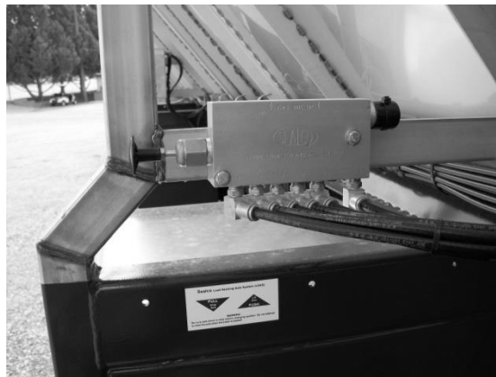
Figure 72 - LSAS Lift Control - Part #003848
