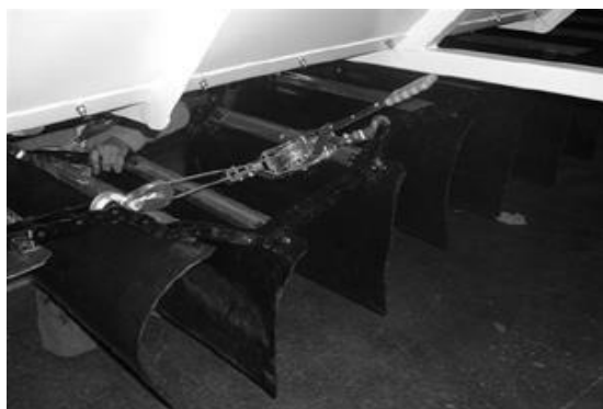
Figure 8 - Using Come-Along To Pull Up Chain Slack
