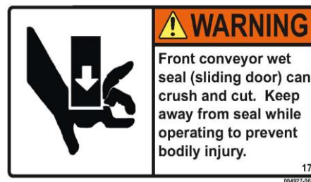
Figure 137- Warning Label for Pneumatically-Actuated Front Wet Seal
