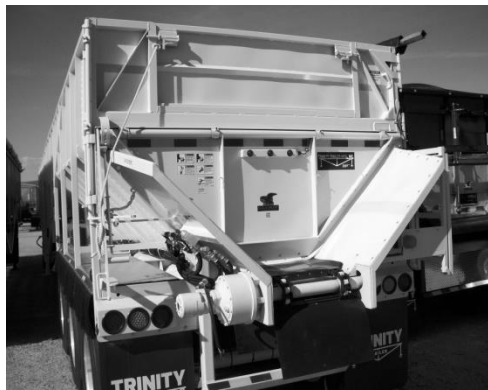
Figure 92- Full Swing "Spud" with manual Flip-Up Door
