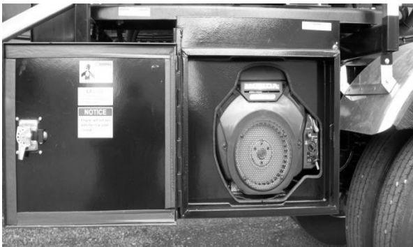
Figure 110- 20 HP Gas Engine (Shown in Optional Enclosure).
