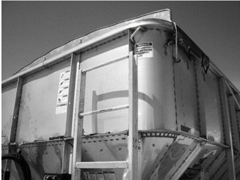
Figure 898 - Front Ladder Showing Upper User Fall Protection Device.
