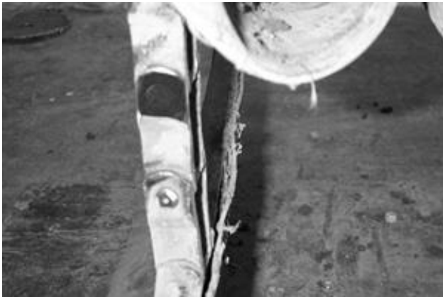
Figure 10- Chain Pin with Head Ground Off
