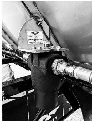
Figure 48 - High Pressure Filter Location
