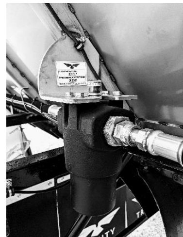
Figure 3- High Pressure Filter Location
