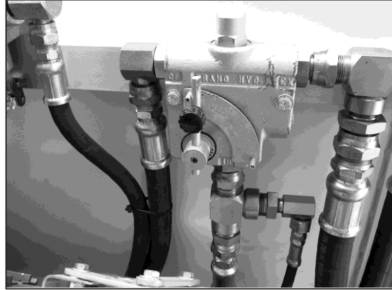
Figure 654- Flow Control Used to Control Belt in PTO Systems. - Part #004402
