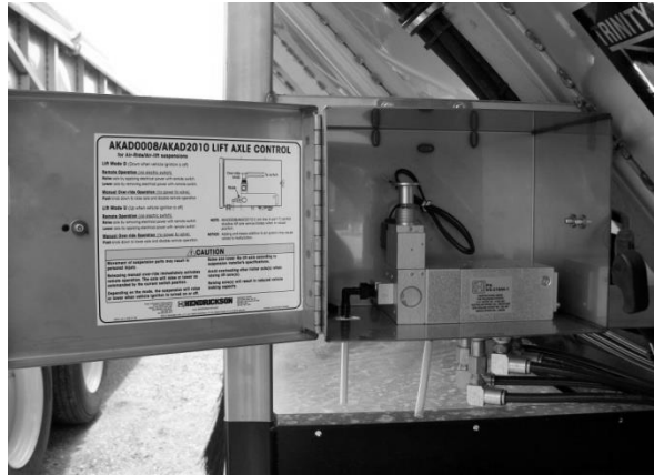
Figure 71 - AKAD2010 Lift Control - Part #004230
