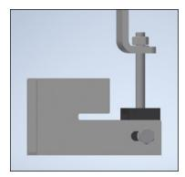
Figure 2 Truck Bed (Open Frame) Mount
