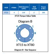
Figure 12 Torque Value and Pattern for Torquing the Pulleys
