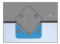
Figure 5 Truck Mount Installed (Blue)
