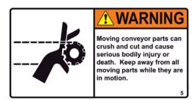
Figure 17 Moving Conveyor Crush Warning
