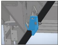
Figure 6 Drill Guide to Complete Closed Frame Mount
