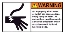
Figure 20 Motor Wiring Decal
