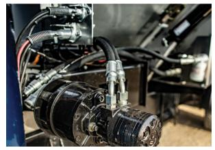
Figure 7 Front PTO & Electric Connections
