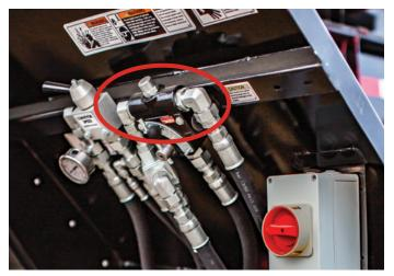
Figure 8 Rear PTO Controls
