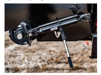
Figure 11 Continuous Belt Adjuster Ratchets
