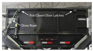
Figure 13 Rear Upper Door Diagram
