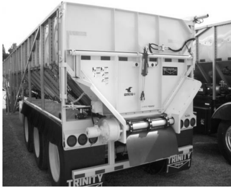
Figure 95 - Full Swing with Hydraulic Flip-Up Door
