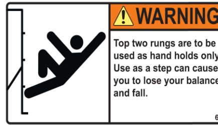
Figure 151 - Top Two Rung Caution Decal
