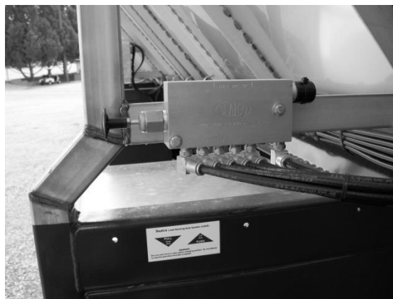
Figure 72 - LSAS Lift Control - Part #003848
