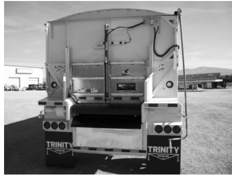
Figure 96 - Full Swing with Hydraulic Slide-Up Door
