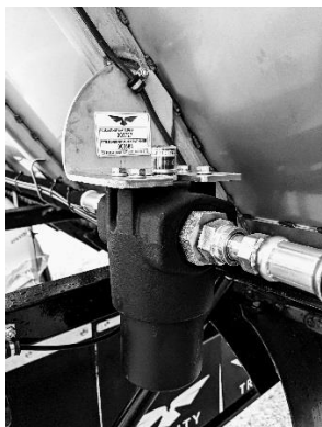
Figure 48 - High Pressure Filter Location
