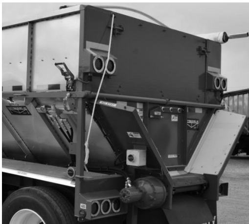
Figure 87 - Manual "Spud" Lower Door.
