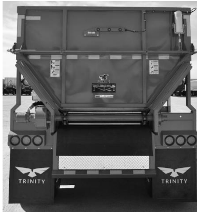
Figure 97 - Hydraulic Lift Top-Hinge with no Lower Door.
