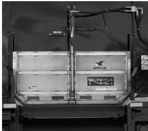
Figure 88 - Hydraulic Slide-Up Lower Door
