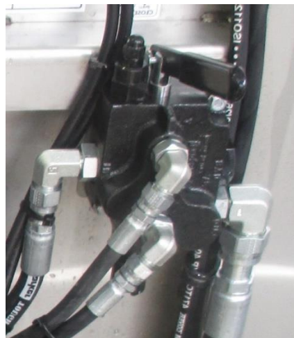
Figure 116 - Single Door Valve for Door Control - Part # 003728
