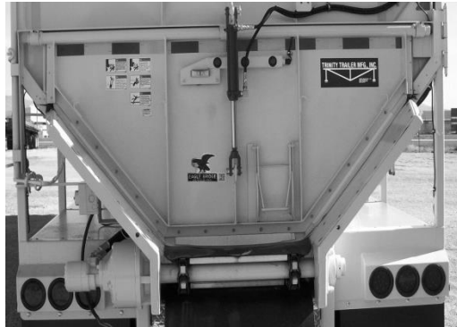
Figure 86 - Hydraulic Flip-Up Lower Door
