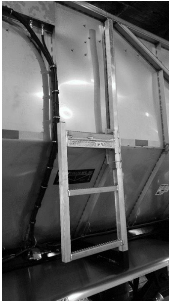
Figure 162 - Maintenance Ladder "Stowed" Position.
