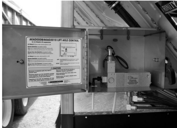
Figure 71 - AKAD2010 Lift Control - Part #004230
