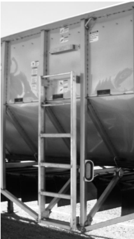
Figure 160- Roadside Ladder Showing Offset
