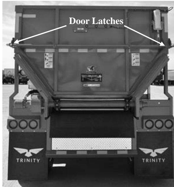
Figure 105 - Top Hinge Pneumatic Latches
