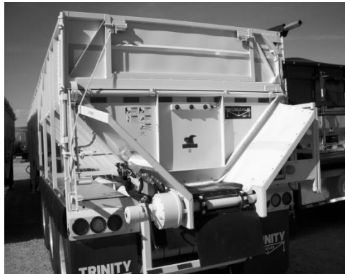
Figure 92 - Full Swing "Spud" with manual Flip-Up Door
