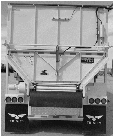
Figure 98 - Hydraulic Lift Top-Hinge with Hydraulic Flip-Up Door
