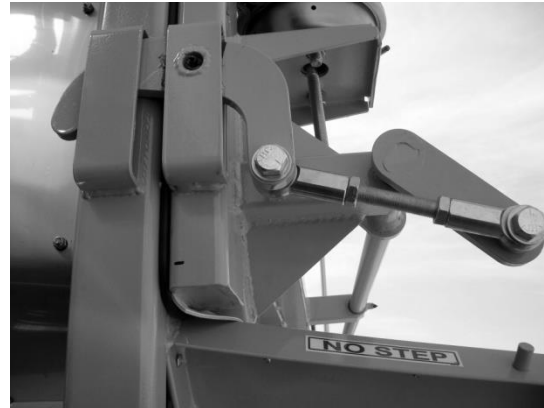
Figure 107 - Top Hinge Pneumatic Latch Disengaged.
