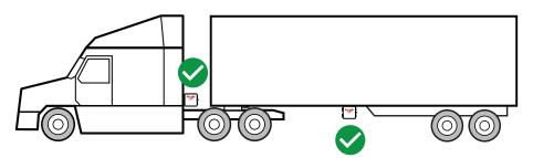
Mount the bracket in the chosen location and install the gauge box to the bracket using supplied hardware.
