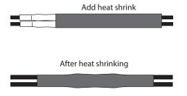
After all connections have been made, heat shrink the entire group of splices so that it seals on the outer jacket of both cables.
