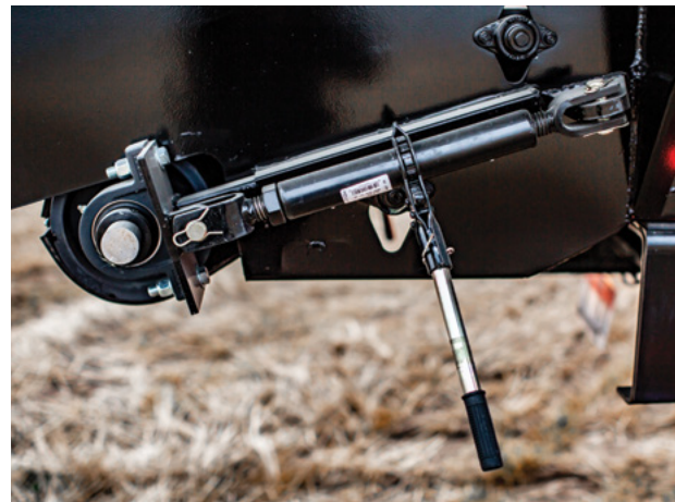
Figure 11 Continuous Belt Adjuster Ratchets
