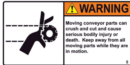
Figure 17 Moving Conveyor Crush Warning
