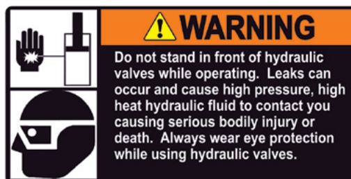
Figure 26 Hydraulic Pressure Leak Warning Label
