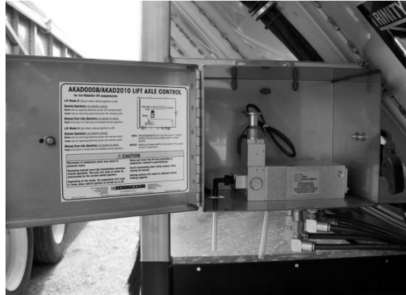
Figure 71 - AKAD2010 Lift Control - Part #004230
