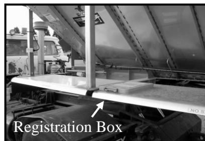
Figure 1- Registration Box (Part # 001675) Location
