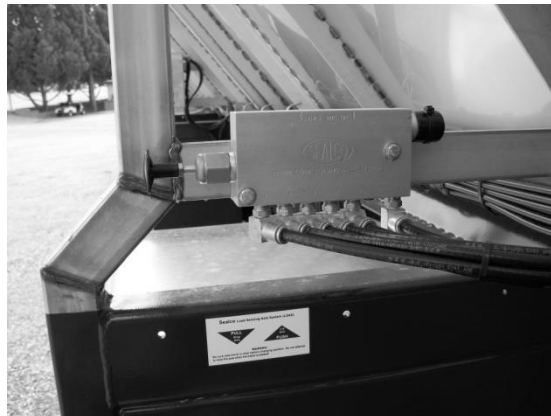
Figure 72 - LSAS Lift Control - Part #003848
