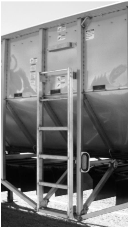
Figure 160- Roadside Ladder Showing Offset
